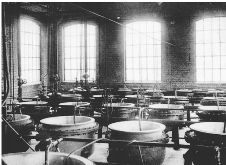
Figure 11-1. Crystallization vats for purifying radium, early 1920s. From Radium (Brussels: Radium Belge [Union Minière du Haut Katanga], 1925), opp. p. 2.
