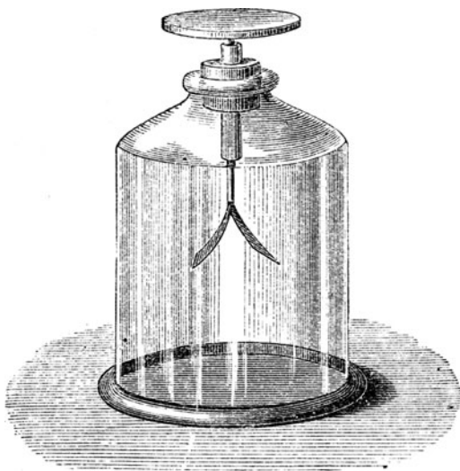
Figure 2-2. Gold leaf electroscope. From Silvanus P. Thompson, Elementary Lessons in Electricity & Magnetism (New York: Macmillan, 1901), 16.
